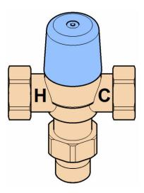
• Attach the sealing ring to the inlet and outlet, and screw the inlet and outlet valve to the mixer. Ensure that the threads are not over-tightened.
